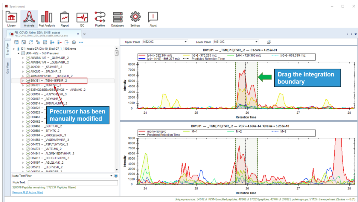
Figure 30. Reviewing Spectronaut peak picking. Integration boundaries can be modified by dragging them. The precursor will be marked as manually modified.
